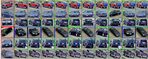
Figure 5. Illustration of vehicle ReID model. The first image is the query image and the other ten images are the 10-nearest neighbors. Green and blue box correspond to the positives and negatives, respectively.
