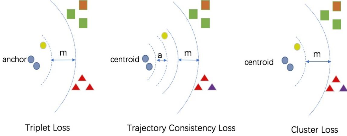
Figure 4. Illustration of different kinds of losses. Different shapes (triangle, circle, and square) represent different classes. The samples with the same color and the same shape are in the same trajectory.
