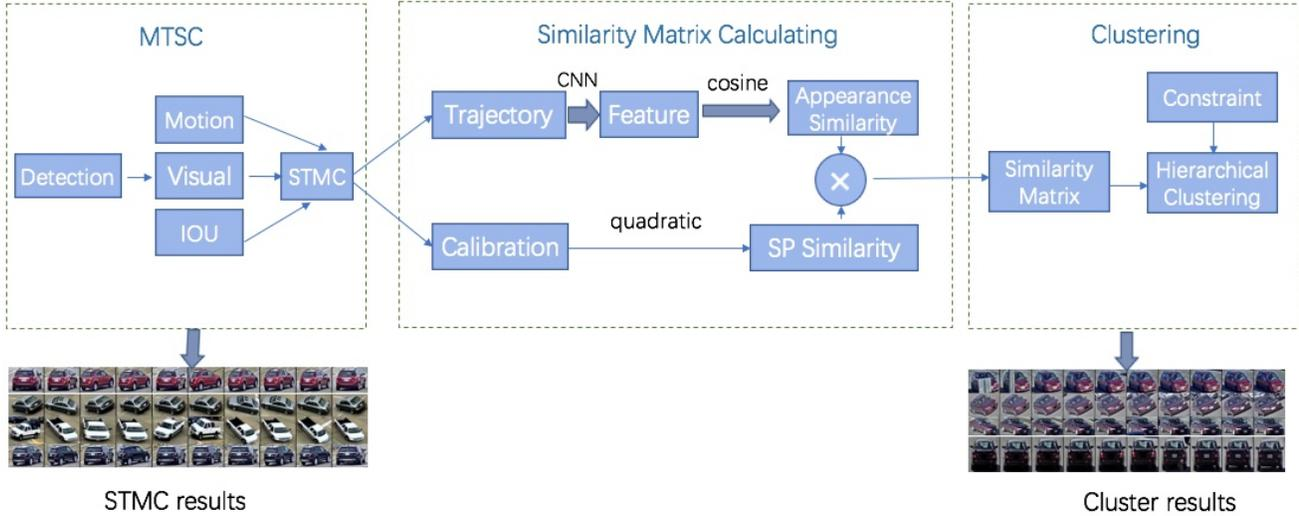
Figure 1. The overall design of our algorithm, which consists of MTSC module, similarity matrix calculating module and clustering module.
