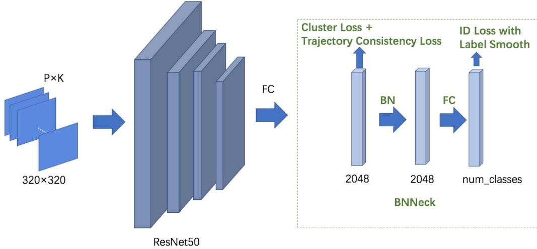
Figure 3. The overall design of the vehicle ReID algorithm, where  $P$  is the number of the ID in the mini batch and  $K$  is the number of images in each ID. The feature before BNNeck is used for cluster loss and trajectory consistent loss while the feature after BNNeck is fed into ID loss.
